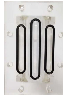
FIGURE 1 (a) A schematic of the experimental setup. (b) A section of the channel. (c) O-rings placed at the end of each channel section for the sealing [Color figure can be viewed at wileyonlinelibrary.com ]
